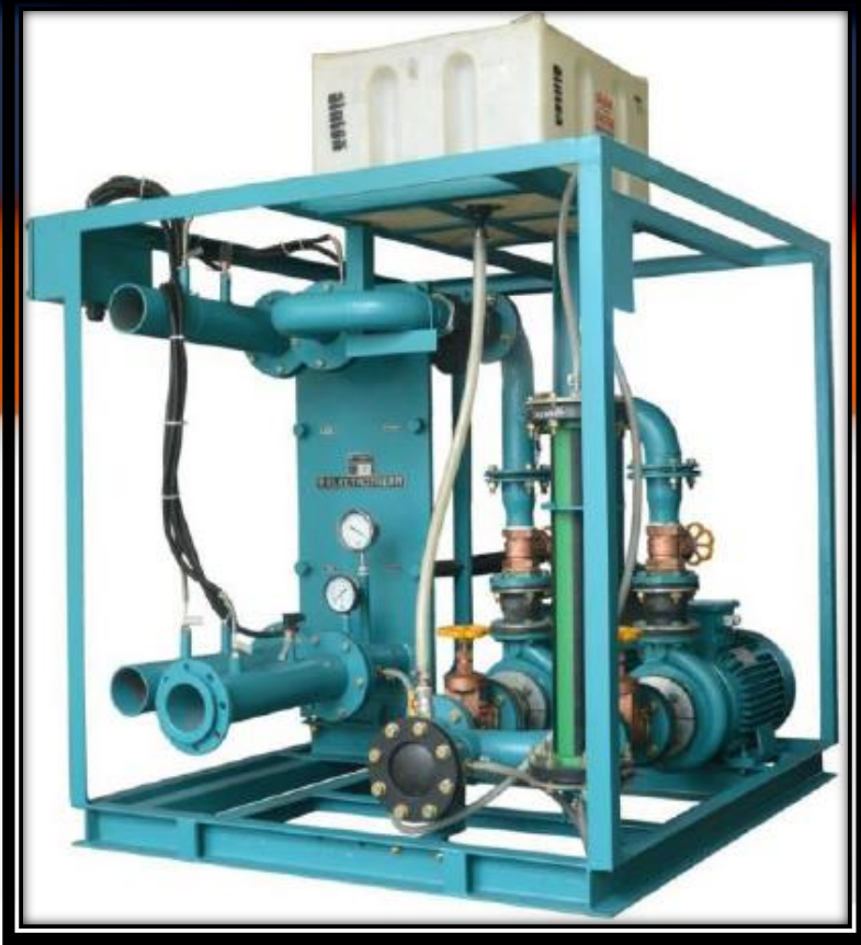
DM Water Circulation System
